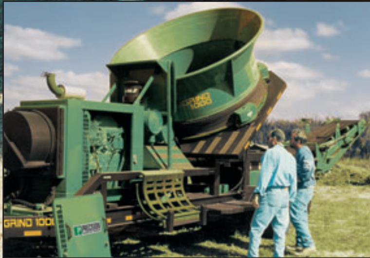
The tub and table tilt forward, providing easy access to the hammermill, auger system and screens.
